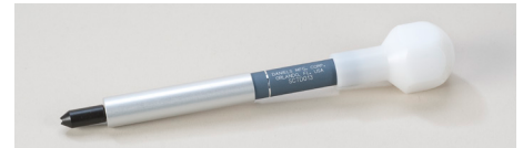
SCTD013 The SCTD013 Push Force Tester is used to apply 2 lbs of force to Safe-T-Cable installations when verifying cable tension on the Torque Verification Blocks (SCT-TB1, SCT-TB1R, and SCT-TB2)
