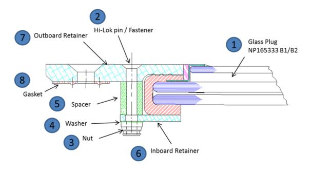
Figure 1 - Plug/Retainer Diagram
