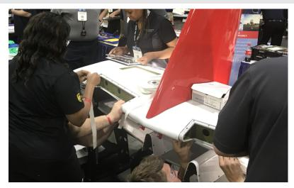
Figure 2 - Teams installing GORE® SKYFLEX® Aerospace Tapes on D-Nose Structure
