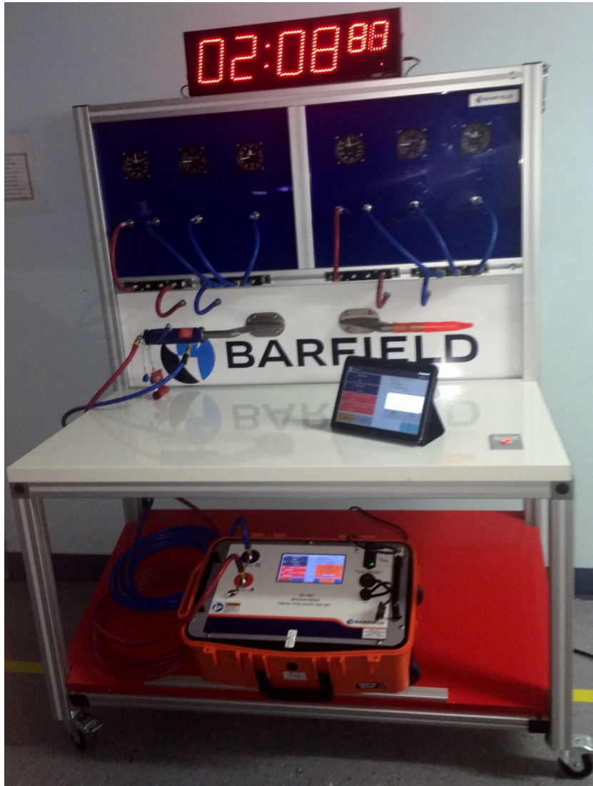
Figure 2 PITOT-STATIC TEST BENCH
